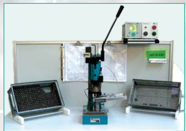
Manual workstation with TPC-MIDI installed on an EP 500-40 toggle press
