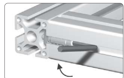
final tightening with socket spanner
