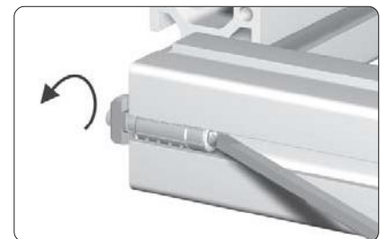
pre-mounting of the T-slot nut
