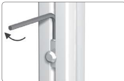
insert and pretension the anchor
