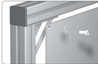
Mounting of cover panels
